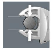
The parallel, smooth jaws of the 7870 Joker offer a seating stress and can thus prevent the nut or screw head from rounding, which can occur when power is transmitted over corners.
